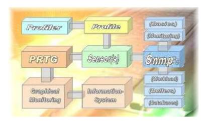
First, the sensor reads out the profile and opens a connection to Snmp via TCP/IP. With the knowledge of IP-Adresss and the Community-Name then Snmp-Devices could be accessed. Then the required function is processed within Snmp and the resulting is transferred back to the sensor. The sensor formats it and divides it to an information-line and channels. This data are transferred then to PRTG.
